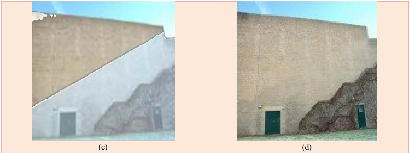
Figure 5. Illustration of shadow removal process: (a) original image, (b) after pixel relighting in YCbCr, (c) after converting to RGB, and (d) after color correction and smoothing
